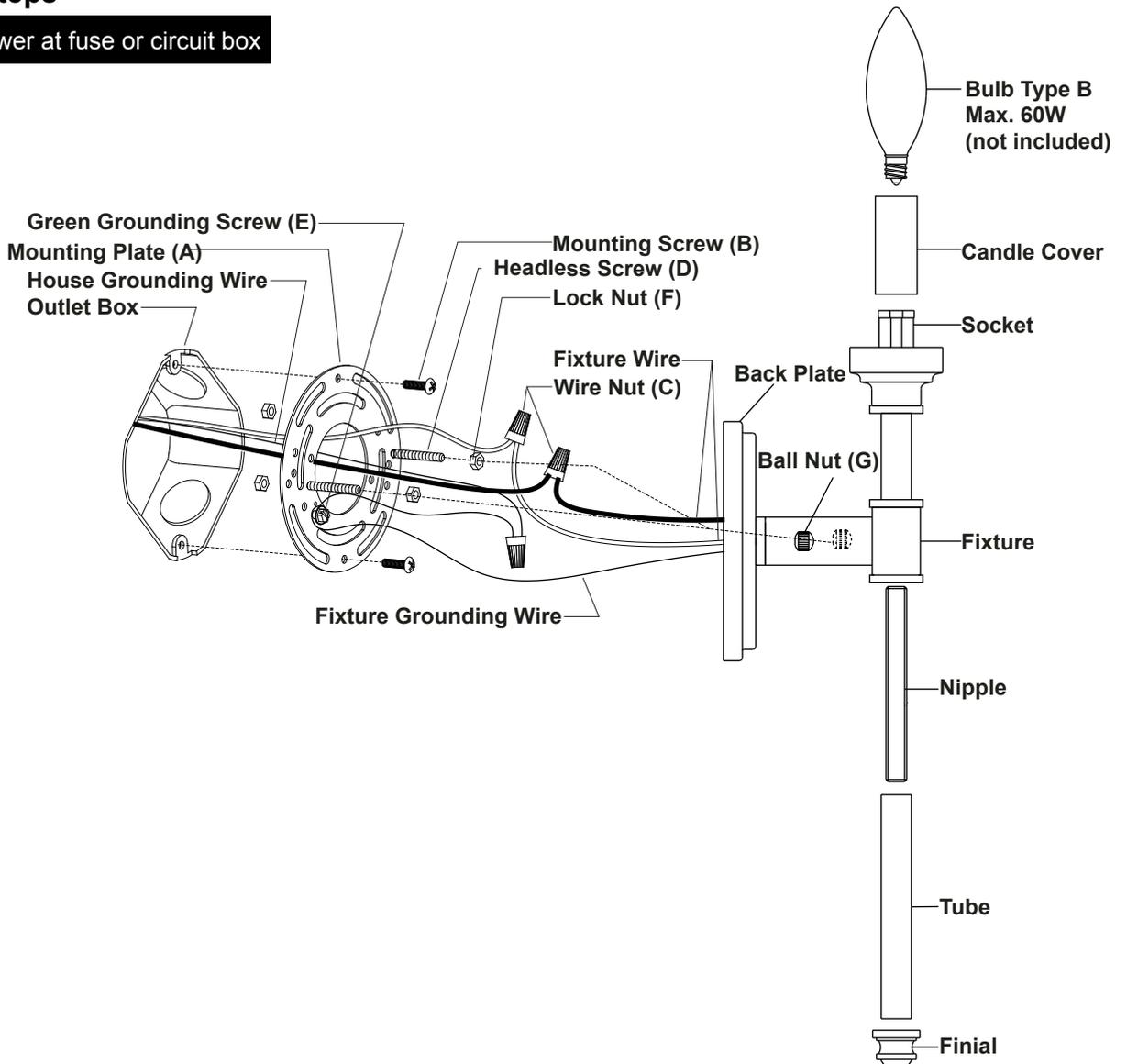
1. Thread two headless screws through the mounting plate, then secure them with four lock nuts (two on each side of the mounting plate). Adjust the length of the headless screws if necessary.
