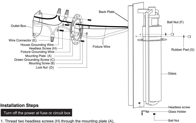
Thread two headless screws (H) through the mounting plate (A), then secure them with four lock nuts (D) (two on each side of the mounting plate (A)). Adjust the length of the headless screws (H) if necessary).
