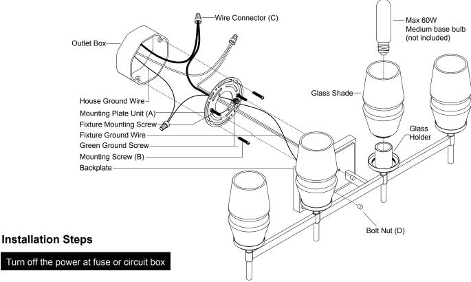
1. Attach mounting plate unit (A) to the outlet box using two mounting screws (B). Adjust the length of the preinstalled fixture mounting screws if necessary.
